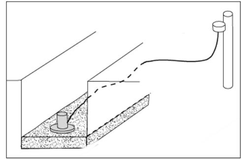
3. Remove sharp stones and rocks and place a 100 mm layer of wet, fine sand on the bottom of the trench.
