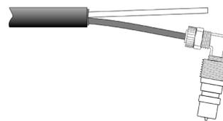
**Tip: If you place the end of the vent tube in a water-filled bottle, the return flow of gas will be visible as bubbles. When the bubbles stop or slow significantly, you can be sure that excess gas has escaped and the transducer is ready to read.**
