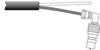
**Tip: If you place the end of the vent tube in a water-filled bottle, the return flow of gas will be visible as bubbles. When the bubbles stop or slow significantly, you can be sure that excess gas has escaped and the transducer is ready to read.**
