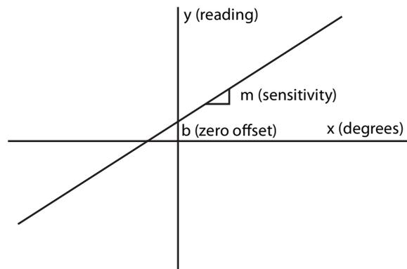
$$\text{Tilt angle} = 1 \text{ degree.} \quad \text{Theoretical reading unit} = 349 \quad (20,000 \times \sin(1))$$
