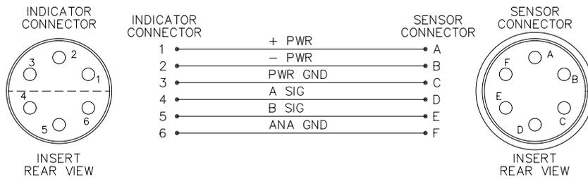
**Testing** Connectors are made to mate with each other but not with any other objects. Never insert the probe of your multimeter into a socket. In making the measurements below, simply touch the probe to the top of the socket.
